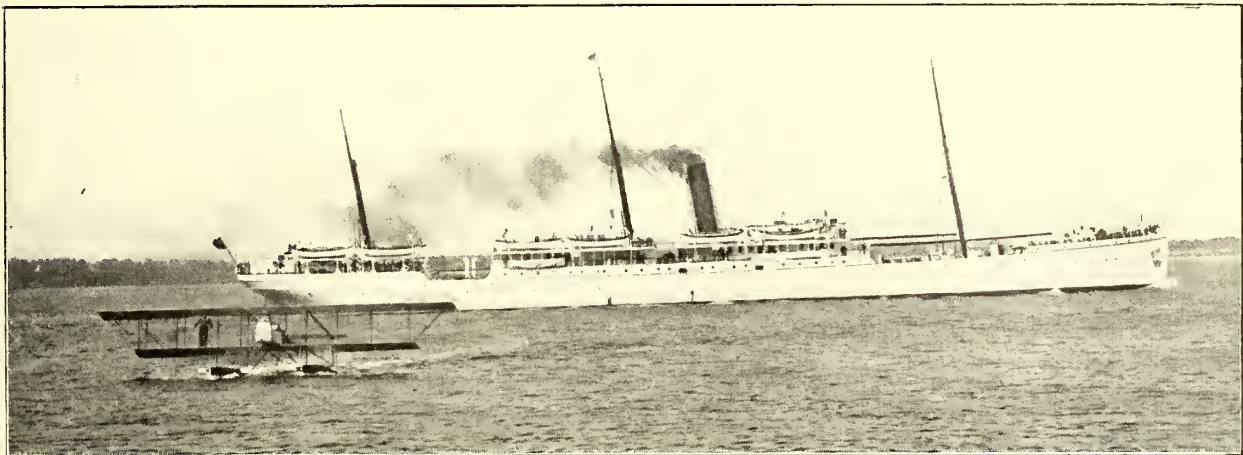
A Maurice Farman taxiing in past one of the South African boats after returning from its trip round the Fleet on Saturday. Note the passenger on the windward wing to keep it down when turning on the water.
